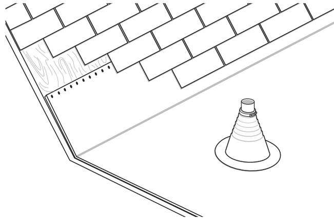
Keep the bottom course of shingles a minimum of four inches (4") above the roof angle change. To adhere the bottom course of loose shingle tabs to the membrane, lift each tab and apply a one inch (1") long bead of *LAP CAULK*.
