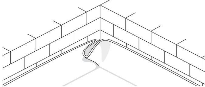
**NOTE:** It is important to adhere the wall flashing on each side of the corner as tightly into the corner as possible. DO NOT STRETCH THE MEMBRANE.
