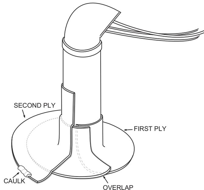
3. Using UNCURED FLASHING, install a six inch (6") wide piece extending three inches (3") up the protrusion and three inches (3") onto the roof deck. Wrap the entire protrusion, allowing a two inch (2") overlap of each flashing. Use as many pieces as necessary to flash the pipe.
