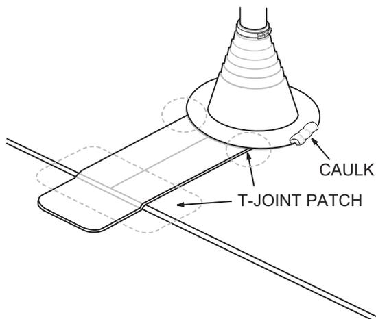
2. Install the pipe boot over the pipe and turn the boot inside out, exposing the bottom of the boot flange. Clean the field membrane at least ten inches (10") in all directions from the pipe. Clean the pipe boot flange and apply *SPLICE ADHESIVE* to both surfaces. Allow the *SPLICE ADHESIVE* to flash off. Pull the pipe boot down, sliding the pipe over the *Water Cut-Off Mastic*, and mating the pipe boot to the field membrane. Hand roll the base of the adhered pipe boot to the field membrane.
