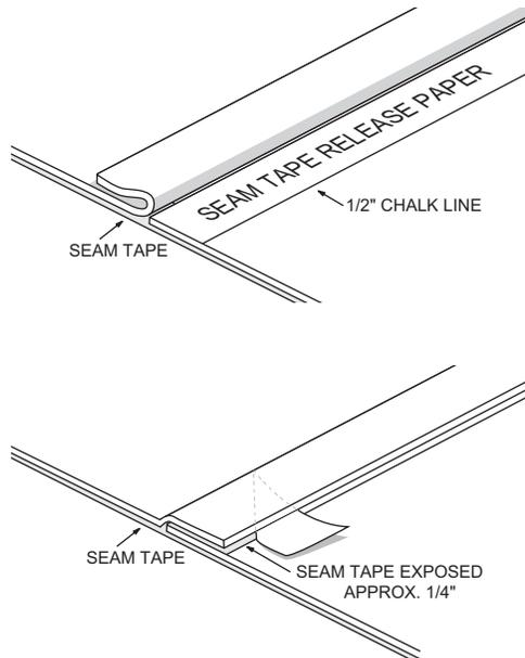
Unroll the Seam Tape along the length of the seam, tape side down, aligning the Seam Tape paper with the marks or chalk line. Using moderate pressure; draw the Scrub Pad along the Seam Tape release paper. This will set the Seam Tape into place and keep air from being trapped under the tape. Fold the top membrane onto the Seam Tape release paper.
