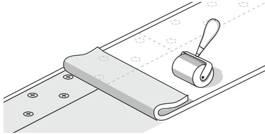
Clean all *Cured* cover strip edges with *Membrane Cleaner* and apply a one quarter inch (1/4") bead of *Lap Caulk* to the seam edges.
