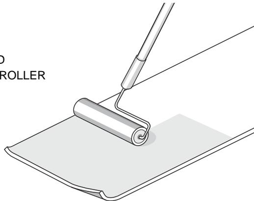
Using *Membrane Cleaner*, clean the metal, the membrane to be seamed, and the Cured Cover Strip. Apply an even coat of Splice Adhesive to the metal drip edge, the membrane area to be seamed, and the Cured Cover Strip.
