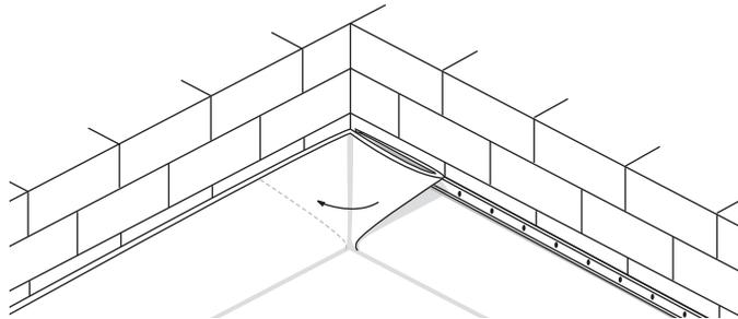
Starting at the base of the inside corner pocket, press the two glued surfaces together. Following standard seaming procedures; adhere the pocket to either wall. Again, following standard flashing procedures, install an UNCURED EPDM (Royal Edge EPDM black, or Re-Flex EPDM white flashing).
