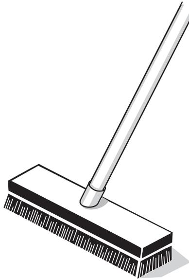
To ensure 100% adhesion of the membrane to the substrate, use a stiff push broom to apply heavy pressure to the fully adhered portion of the sheet. DO NOT apply enough pressure to cause the RPI membrane to wrinkle. Fold back the remaining unglued portion of the sheet and repeat the process. Install adjoining sheets so that water flows OVER, and not against, the over-lapping edges.
