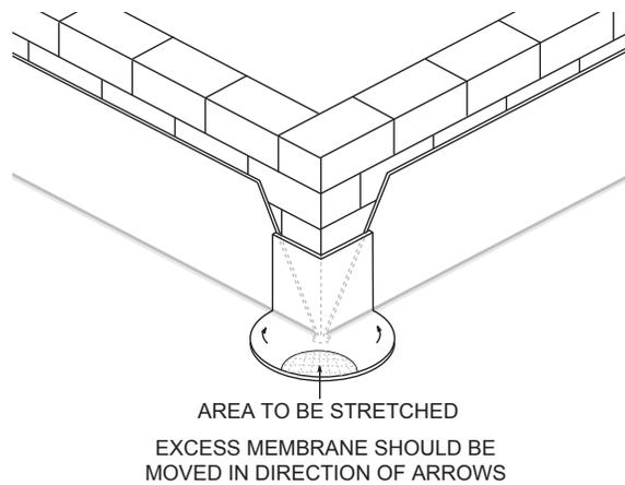
5. Beginning at one inside angle change, adhere the flashing into the angle and approximately one inch (1") onto the roof. Before the membrane can be adhered to the other angle change and onto the roof, it must be stretched. Do not stretch the membrane at the angle changes or base of the outside corner (fig. 3.oc) All stretching should be done to the membrane as shown in (fig. 3A OC), stretching the middle of the flashing towards each corner as the flashing is mated to the field membrane.
