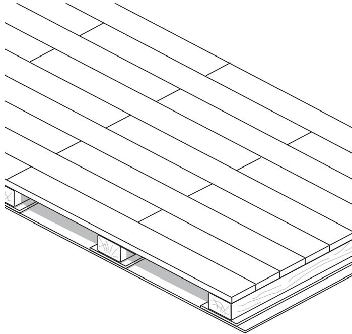
DO NOT attach the sleepers through the membrane. The deck should be secured at a side wall, post, or perimeter area. When attaching outdoor carpet, use an exterior grade latex based carpet adhesive according to manufacturer's instructions.
