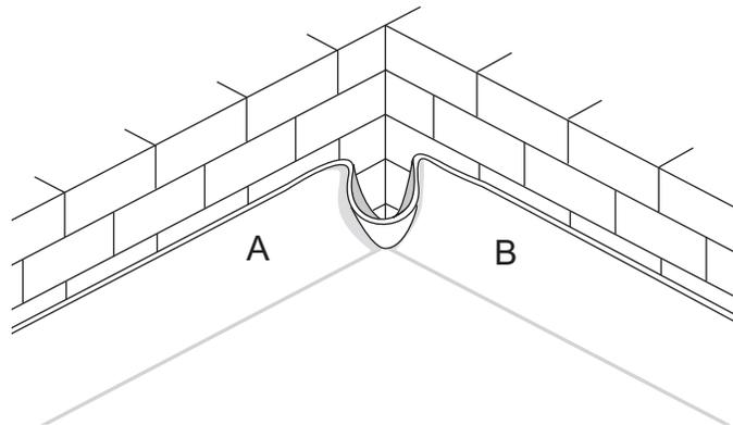
After one side is flashed in, (A), begin the other side, (B). When both walls are flashed in, all excess material should form a pocket in the corner.
