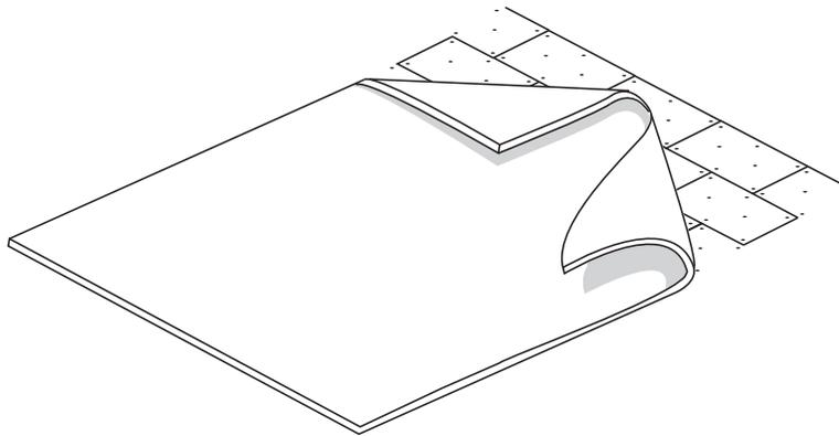
**NOTE:** When a protrusion is encountered (i.e., pipes, skylights, etc.), cut the field membrane from the nearest seam (edge) to allow the sheet to roll around the protrusion with the least possible cuts. Once the field sheet has been fully adhered into place, flash over the cut with a piece of RPI Royal Edge or RPI Re-Flex EPDM/TPO Cover Tape. When using Cover Tape, always use appropriate Primer. The flashing should extend a minimum of three inches (3") on each side of the cut.
